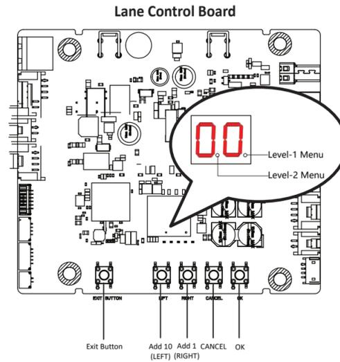
The buttons and the display screen are on the lane control board.
